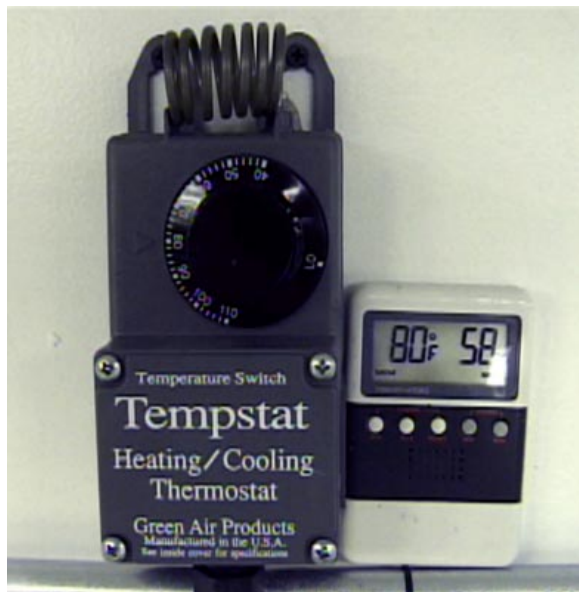
A basic thermostat (left) to control the temperature. A thermometer and humidistat (right) indicate the temperature is 80 degrees Fahrenheit and the humidity is 58 percent. As you can probably tell from the design, these are two separate units. More expensive models measure and control everything all in one unit.
